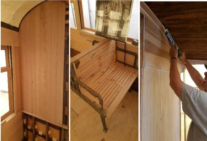
While waiting for the seat frames we continue work of the coupler pocket mountings. These have turned out to be a challenge with alignment of existing mounting holes. Along with that we are caulking the exterior in preparation for painting. Soon work will start on the roof. Please take a moment when you are at the museum to come back and see the car first hand. It is truly an impressive sight!
