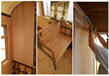
While waiting for the seat frames we continue work of the coupler pocket mountings. These have turned out to be a challenge with alignment of existing mounting holes. Along with that we are caulking the exterior in preparation for painting. Soon work will start on the roof. Please take a moment when you are at the museum to come back and see the car first hand. It is truly an impressive sight!
