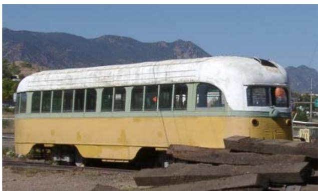
Except for the air compressor, everything in Car No. 3101 is original. A DH-16 air compressor, taken off an older car during the war, replaced the original air compressor which failed early on.
