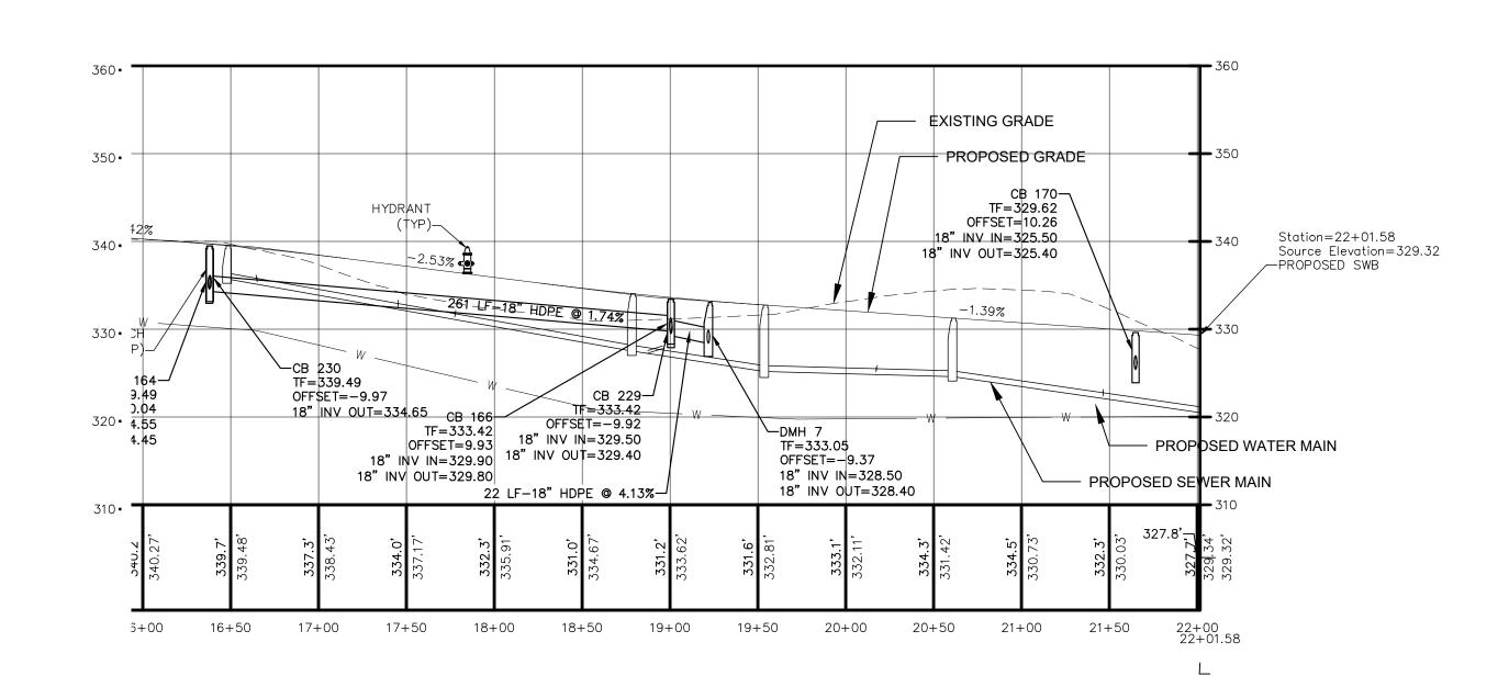
WATER MAIN TO BE 5' BELOW FINISHED GRADE MIN. VERTICAL SEPARATION OF 1.5' FEET MINIMUM BETWEEN SANITARY MAIN AND SERVICE LINES AND BETWEEN STORM MAIN.
