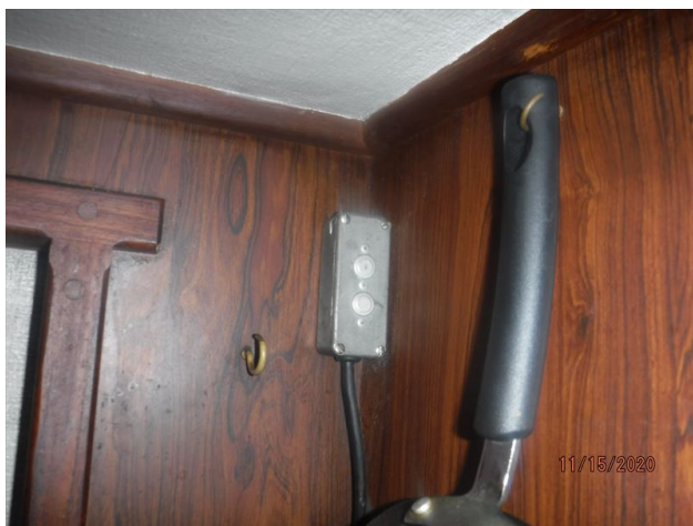
BILGE HIGH WATER ALARMS Two (2) Bilge High Water Alarms. Test sounded.
