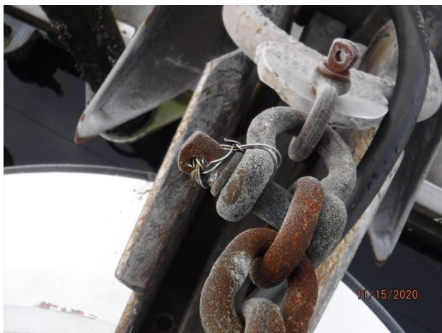
RIGGING CLEVIS PINS & COTTER PINS Appeared serviceable moused as per good marine practice
