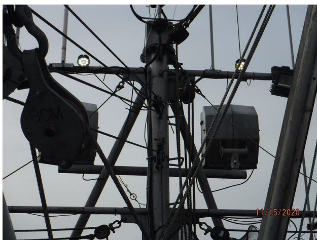
RIGGING CLEVIS PINS & COTTER PINS Appeared serviceable moused as per good marine practice
