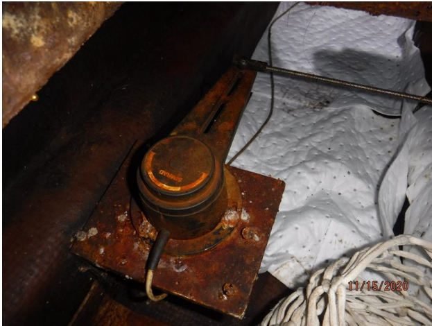
RUDDER INDICATOR DIAL Two, one at each helm station
