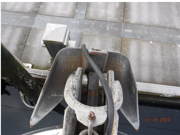
ANCHOR RODE TYPE 1/2" Galvanized chain is full on the winch
