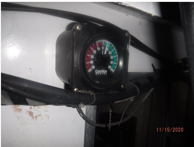
RUDDER INDICATOR DIAL Two, one at each helm station
