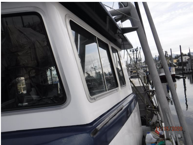
WINDSHIELD Tempered glass windshield with aluminum frame by Diamond SeaGlaze and 12vdc wipers
