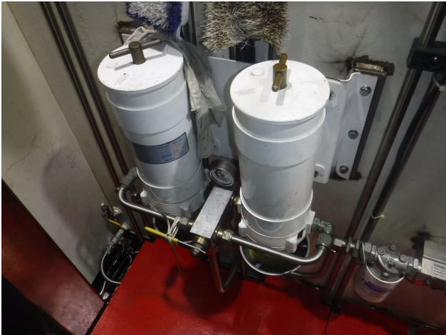
MAIN ENGINE SECONDARY FUEL FILTERS Engine mounted Secondary Fuel Filters.
