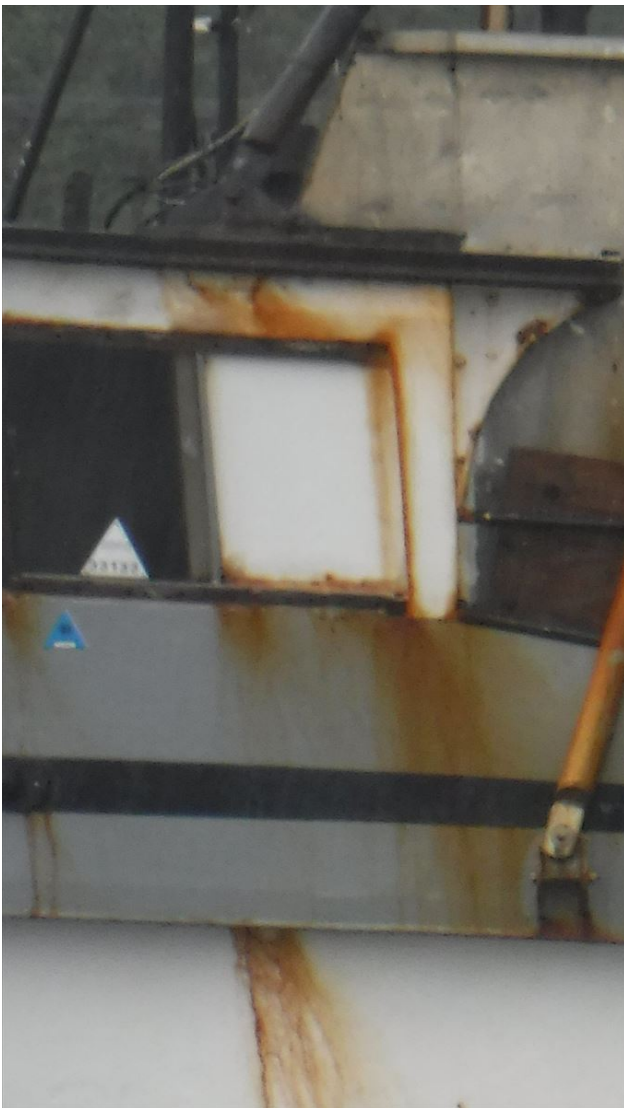
TRANSOM Steel bulwark capped with stainless grab rails
