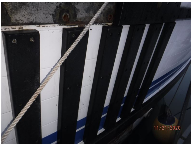
HULL-TO-DECK JOINT TYPE Appeared to be an internal flange type joint.
