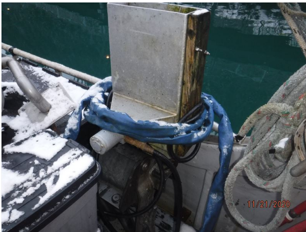
BAIT HANDLING Hydraulic chopper
