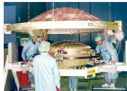
Figure 2: Huygens Entry Assembly Module and Descent Module
