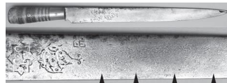
Figure 4: The close-up of this blade shows the kirk narduban (Mohammed's ladder) pattern with several 'rungs' (above arrows) oriented perpendicular to the length of the blade representing an induced alteration in the background pattern. (Photo credit: Lee A. Jones.)
