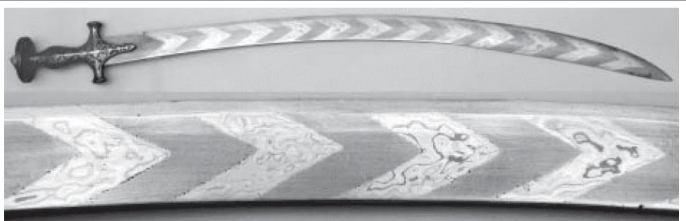
Figure 5: Details of an Indian chevron patterned talwar, likely 19th or 20th century. Clearly made for show, but fully serviceable if the welds are well made.
