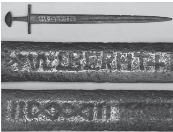
Figure 4: A European sword of the mid to late Viking Age, mid 10th to early 11th century, bearing a variant of the +ULFBERHT+ inscription on one face of the forte and a geometric pattern on the opposite face. The inlay is composed of twisted rods made from stacked steels of varying composition likely forged into grooves in the face of the blade and then dressed flat. Though contemporary with the Vikings, the brazil nut pommel suggests mounting nearer the origin of the blade, speculated to have been in what is now Germany. The steel surrounding the inscription has been brightened by polishing to increase contrast.
