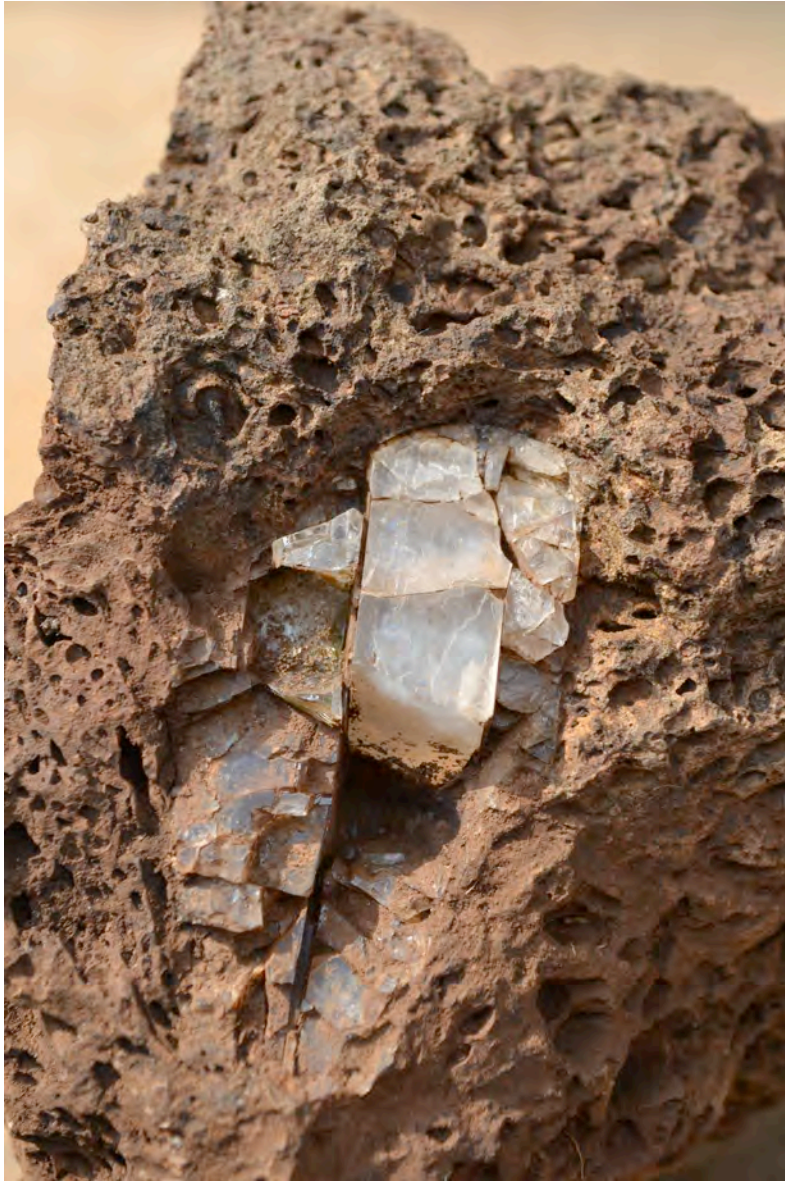
Fig. 3. Gem-quality anorthoclase (9 cm) in mugarite from Sovann Kriri Vattana Ram Ting Jak monastery, Ratanakiri province, Cambodia.
