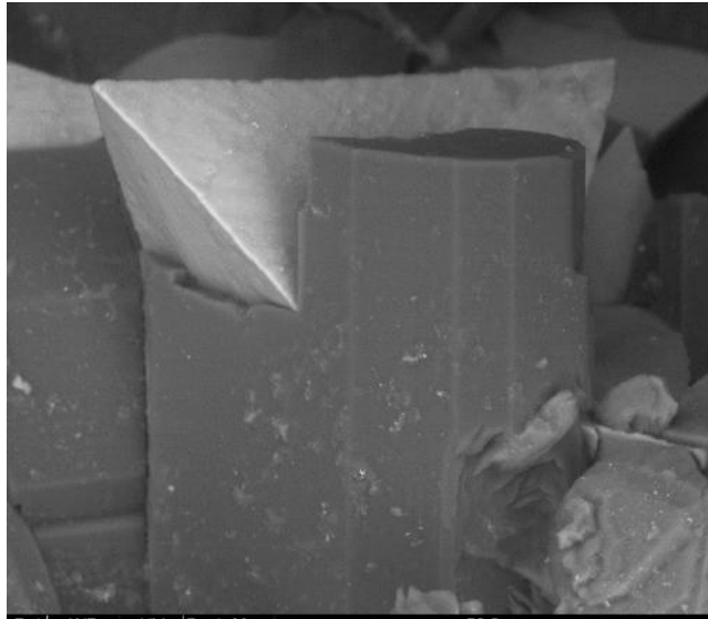
Figure 1. SEM micrograph of bertrandite (dark color) and genthelvite (lighter color) from the St. Peters Dome area.
