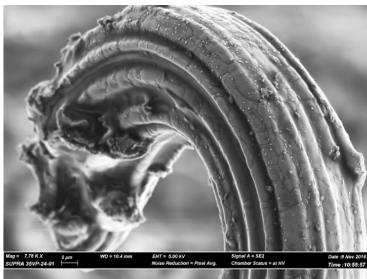
Figure 2: SEM image of a synthetic wire silver shows striations superimposed on a roughly equigranular texture.
