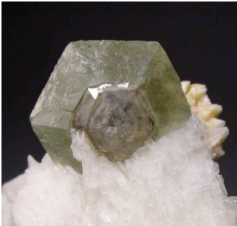
Figure 1. A 1 cm bipyramidal crystal of zoned hydroxylapatite (green) and fluorapatite (grey core) on albite from the Sapo mine.
