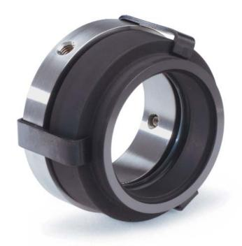
The AST 50 Mechanical Seal is readily accessible, not hidden in the stuffing box, so it's easy to install and replace. Since the proper spring compression is preset, there are only three steps to installation. Just slide the rotary unit over the shaft until it comes in contact with the stationary face, tighten the drive ring to the shaft, and remove the retaining clips.
