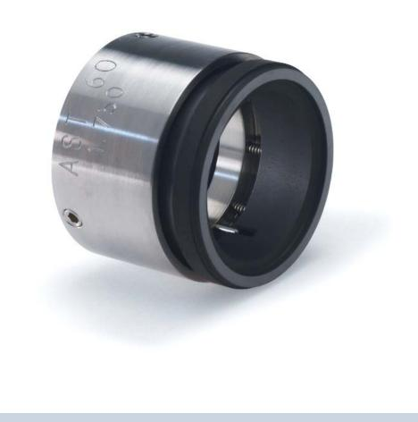
The AST 60 is a simple and easily installed seal that can be used wherever a highly reliable, anti-clog seal is needed. Its narrow seal face design and hydraulic balance make it a cool-running seal. The floating rotary seal ring eliminates seal face distortion inherent to shrink fit designs. Since all the springs are isolated from the pumped fluid, flush rates can be reduced to minimize product dilution.
