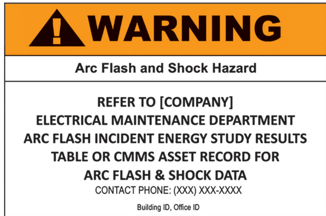
Figure 1: Alternate Equipment Label — Arc Flash Data Provided In Results Table
