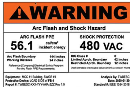
Figure 2. Warning Signal Pane Arc Flash & Shock Equipment Label
