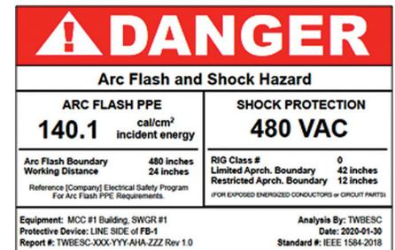
Figure 3. Danger Signal Pane Arc Flash & Shock Equipment Label (incident energy ≥140 cal/cm<sup>2</sup>)
