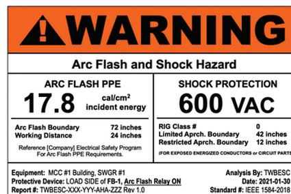
Figure 5. Warning Arc Flash & Shock Equipment Label Arc Flash Relay ON
