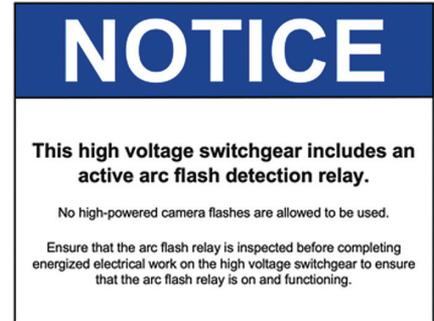
**Figure 9.** Notice Signage Arc Flash Relay Installed
