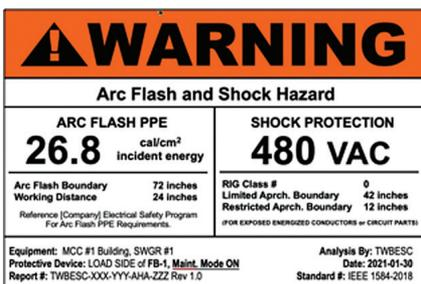
Figure 4. Warning Arc Flash & Shock Equipment Label Maintenance Mode ON
