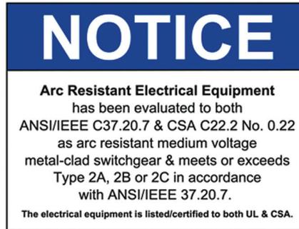
**Figure 8.** Notice Signage Arc Resistant Electrical Equipment
