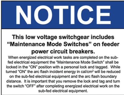
**Figure 7.** Notice Signage “Maintenance Mode Switches”
