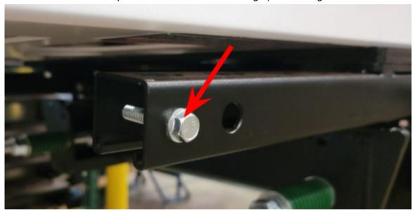
12. Re-lock the pull pins by pulling out and twisting them. Then push the conveyor forward into place as shown below.
