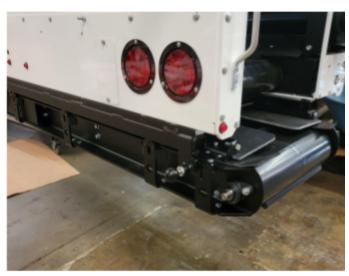
8. Re-install and tighten the stop plates onto both sides of the conveyor.
