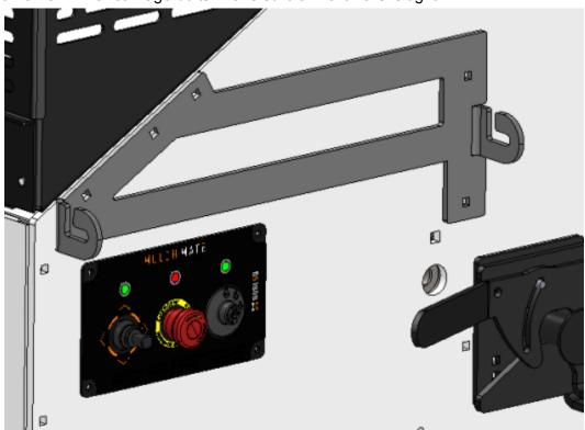
2. Mount the extension conveyor rails to the bottom the the Mulch Mate using the (8) %-16 x 1.5" flanged hex bolts.To not fully tighten until after all 8 bolts are installed.
