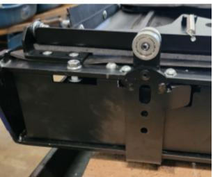
6. Make sure the pins shown below are pulled out and locked. This is done by pulling them out and twisting them 90 degrees.
