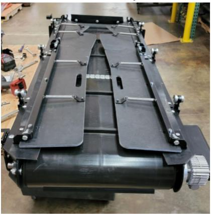
4. Remove the stop plate shown below from the motor side of the conveyor
