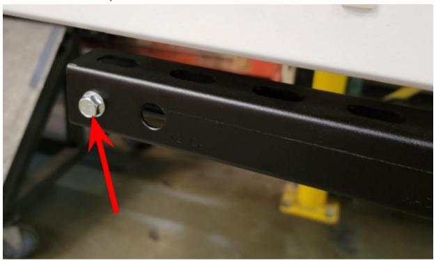
10. Push the conveyor back until the bolt shown below is past the track and re-install the back bracket previously removed. Make sure installed bracket has ½" gap off side rail.
