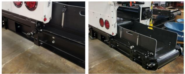
4. Before fully pulling out the extension conveyor, attached the cam straps to the front bearing bracket hole
