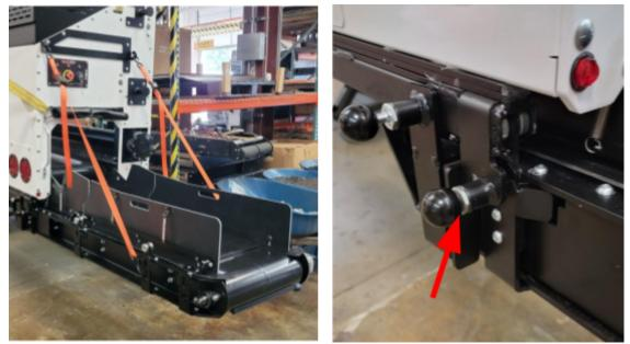
6. From the fully pulled out position, the angle of the extension conveyor can be adjusted by lifting the conveyor and tightening the straps to the desired height. This can add up to 15" of extra height for dispensing material.
