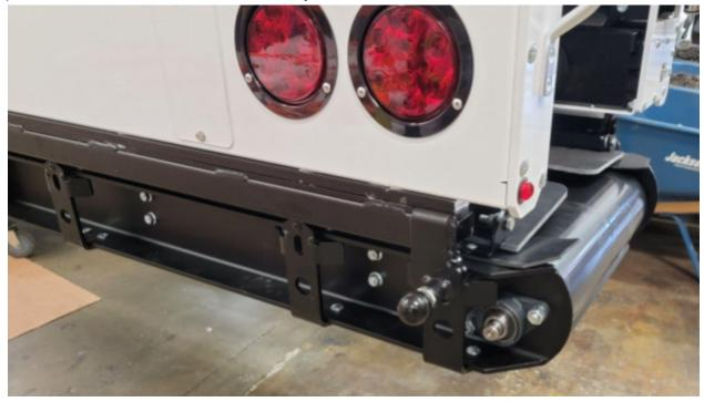
2. If you want to use the Mulch Mate with a wheelbarrow and do not want to use the extension conveyor, you can slide the conveyor back further and lock it with the rear locking bracket in the hole at the back of the track system.
