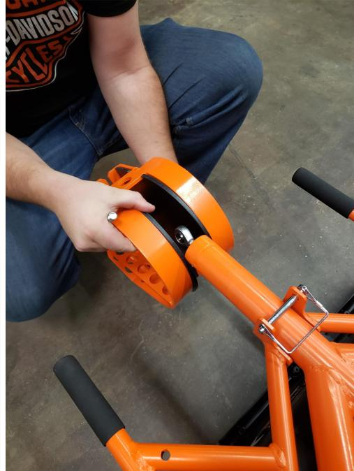
8. Insert  $\frac{5}{8}$ " bolt through the knuckle and ball joint. Tighten down with  $15/16$ " socket & wrench.
