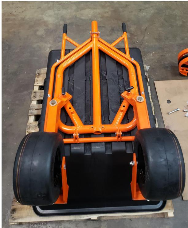
6. Install ball joint rod end. Make sure to leave between  $\frac{1}{4}$ " and  $\frac{1}{2}$ " of thread exposed.
