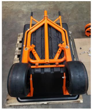
6. Install ball joint rod end. Make sure to leave between  $\frac{1}{4}$  and  $\frac{1}{2}$  of thread exposed.
