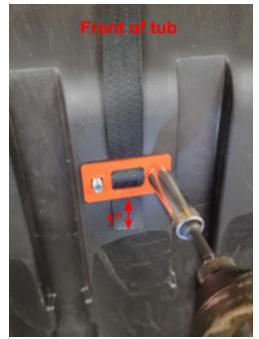
12. Install the 2 bolts in the holes drilled in step 3 so that the head of the bolt is on the inside of the tub. Tighten down the nuts onto the bolts so that the shoulder of the bolt head is pulled into the plastic.
