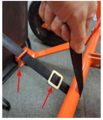
22. Wrap the nylon strap around the kart mate frame the double dump arms are bolted to, and thread the strap back through the bracket as shown below.
