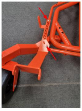
17. Place the tub onto the frame and install the 3/18-16 hex bolts through the double dump arms and the pivot brackets
