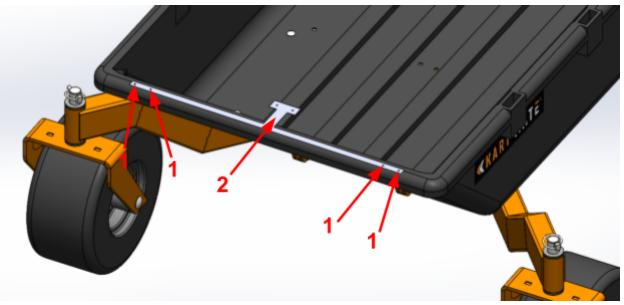
3. Fold down the tab in the center and drill out the 2 holes on the tab with a <sup>1</sup>/<sub>8</sub>"drill bit.
