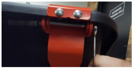
19. Tighten the nuts installed in step 16, holding the double dump arms to the kart mate frame.
