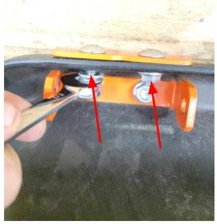
10. Install the plate and bolts inside the tub as shown below
