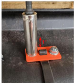
14. Install the handle bracket in the holes drilled in the back of the tub. Make sure the head of the bolts are underneath the tub and the nuts inside of the tub.
