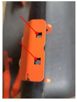
9. Install and tighten the carriage bolts in the holes drilled in the previous step
