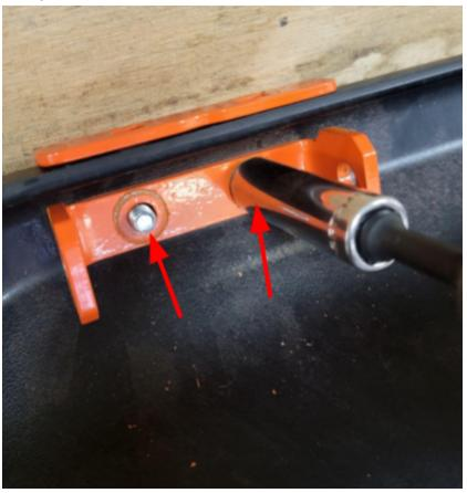
8. Drill out the front 2 holes to 5/16" on the bracket installed in step 6.
