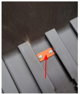
11. Thread the nylon strap through the bracket shown below so that about an 1in of material sticks out. Bolt the plate underneath the tub sharing the bolts of the plate installed in the previous step. Make sure the long end of the strap sticks out towards the front of the tub.
