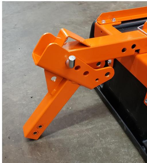
11. Flip everything over and insert Kart Mate into the front hitch mount on the mower.
