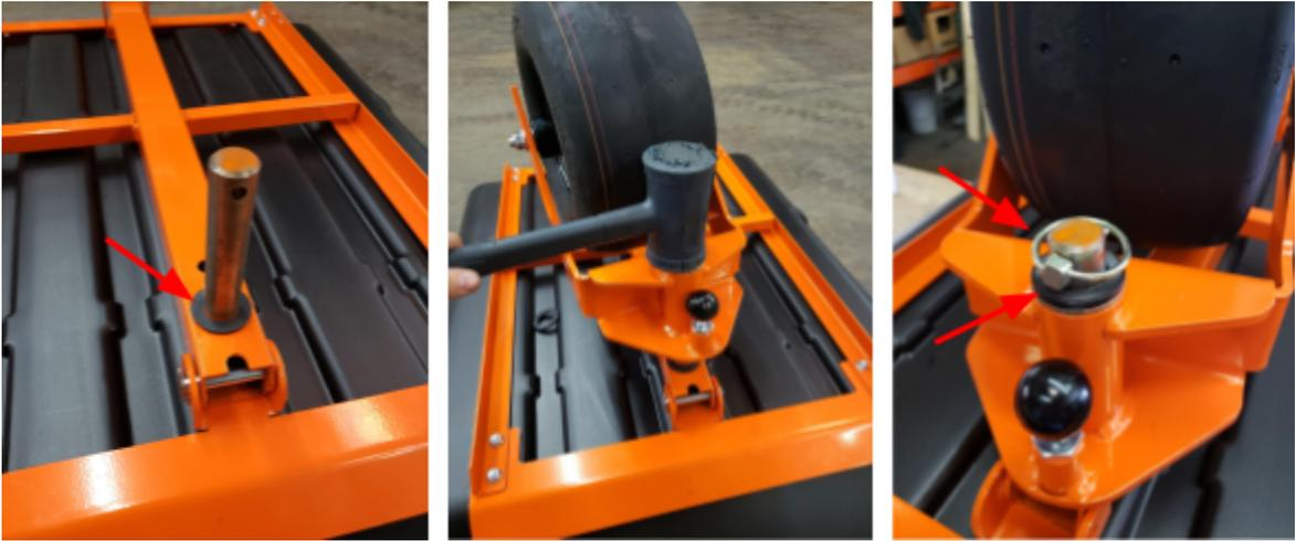
10. Install the knuckle to the back side of the main frame assembly with the provided  $\frac{5}{8}$ " hitch pin.
