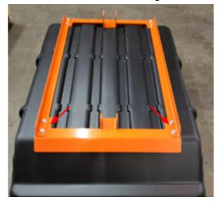
6. Install the 1x1 tube into the main frame assembly and bolt together using the 5/16-18 x 1.75 carriage bolts. Make sure the square holes in the 1x1 tube are facing up.
