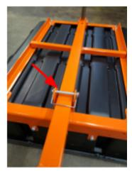
8. Make sure the main frame assembly is centered on the tub. Tighten down all of the nuts with a ½" socket and impact until the head of the carriage bolts sit flat on the inside of the tub.
