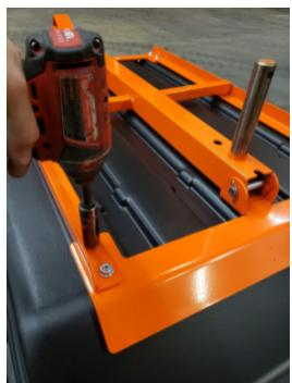
9. Install 1 plastic washer onto the shaft. Slide and rotate the caster assembly onto the shaft. If needed use a rubber mallet to assist. Install 2nd plastic washer over the caster assembly and insert linch pin thru hole in shaft.
