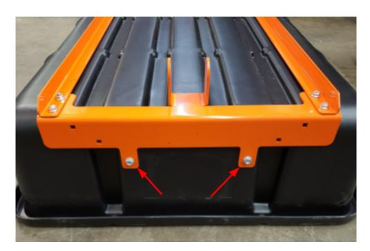
5. Place the front bracket on the tub and install the 4 carriage bolts thru the tub and the side rails/front bracket. Hand tighten nuts.
