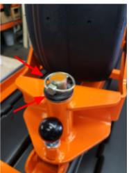
10. Install the knuckle to the back side of the main frame assembly with the provided %" hitch pin.
