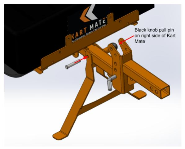
Install leg assembly onto frame and insert pin through holes in leg and frame.
