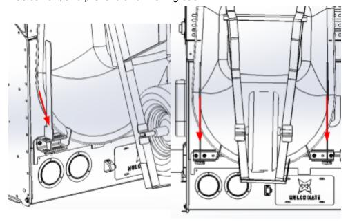
• Secure upright support with lynch pin in the hole at the bottom
