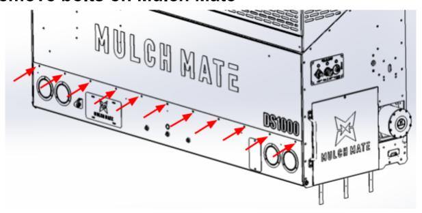
To access the outer bolt on each side, 2 panels from inside the machine need to be removed..
