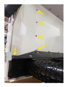
2. Gently pull back the black clip and separate the connector from the control panel above the "SEPD" module. Remove the four #30 Torx screws on the control panel and replace the control panel. Reconnect the harness until it clicks in place. It can only go in one way. Test unit by turning on power, activate to get 2 green lights and press down on the joystick. When you press joystick you should see
