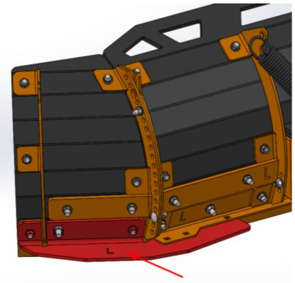
9. Loosely Install the two <sup>3</sup>/<sub>8</sub>-16 x 1in long carriage bolts and nuts as shown
