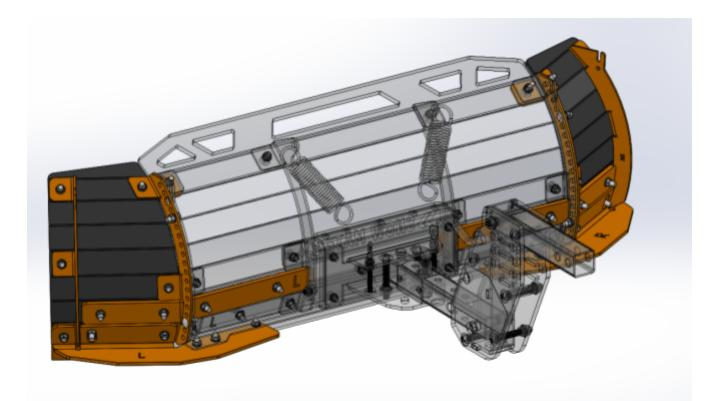
1. Slide the wing support bar into each of the winglet assemblies. And loosely bolt them down with the  $\frac{3}{6}-16 \times 1.5$ " Carriage bolts.
