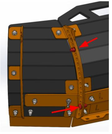
5. **Loosely** bolt the support bar to the main plow assembly using the <sup>3</sup>/<sub>8</sub>-16 x 1.5" carriage bolts.
