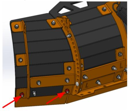
8. Install the reinforcement bracket as shown and **loosely** reinstall the nuts removed in the previous step.
