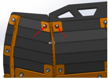
11. Install the top connecting bracket so that the rectangular hole is on the winglet side, the square hole is on the main plow side, and the bracket is angled up. Note there is a left bracket and a right bracket. Make sure you have the correct one. Reinstall the nuts and bolts removed in the previous step.
