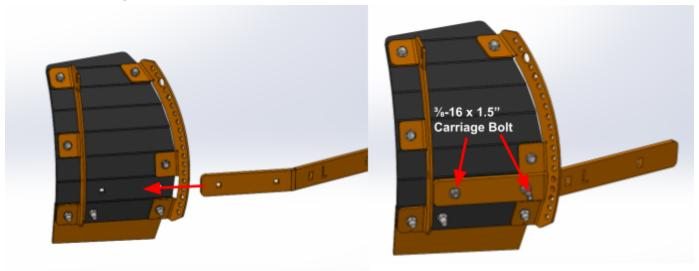
2. Loosen (do not remove) the 3 nuts on each of the outside main plow support brackets
