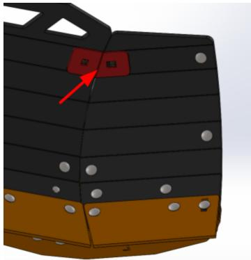
12. Tighten all of the nuts on the winglet and main plow.
