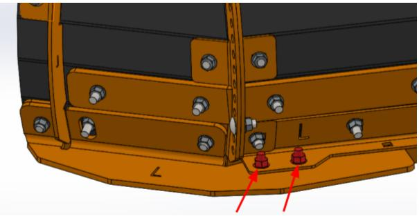
10. Remove the 2 nuts and bolts at the top of the winglet and snow plow as shown below.
