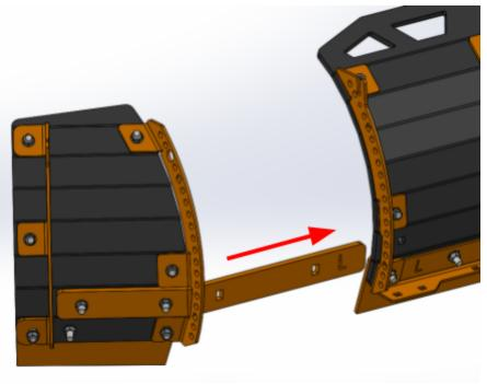
4. Loosely bolt the support brackets together using the 3/8-16 x 1" carriage bolts
