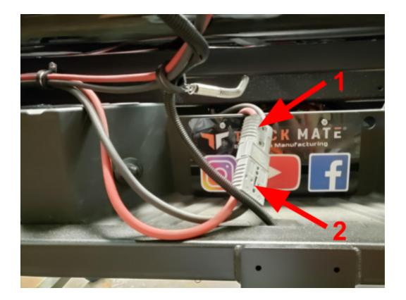
Plug smaller Anderson connector coming from Truck Mate motor to smaller Anderson connecter mounted to the back of the conveyor assembly
