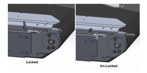
With the help of a second person. Pick up the conveyor assembly and install it onto the tarp tube, between the black plastic guides on the tube, and then push the conveyor up all the way until it latches in place.
