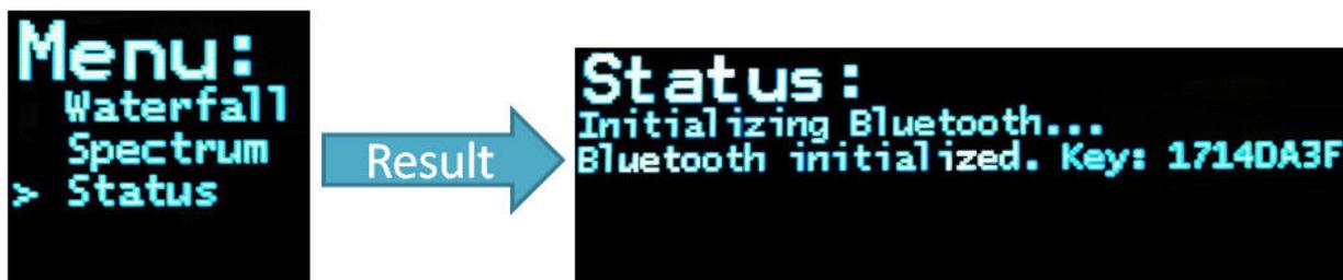
Figure 9: The Bluetooth pairing key
