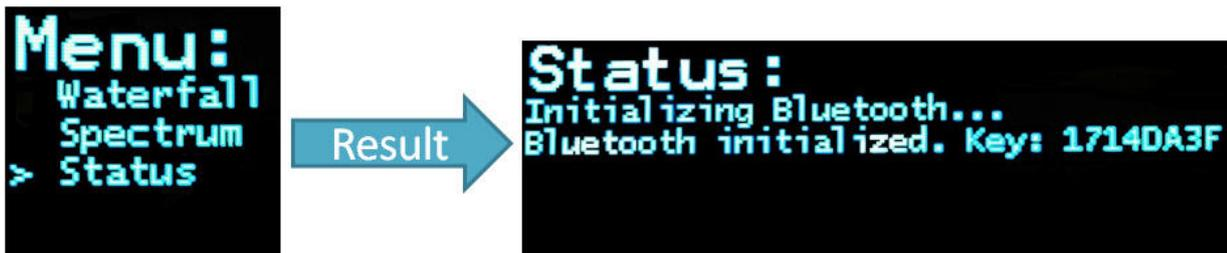
Figure 9: The Bluetooth pairing key
