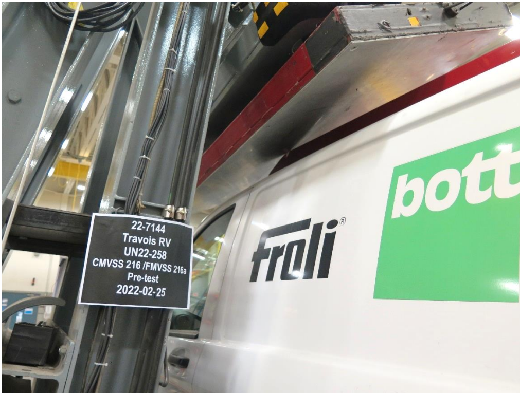
11. Rear view with test device aligned at initial contact point – pre-test
