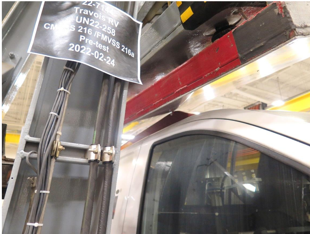
17. Front view with test device aligned at initial contact point – pre-test
