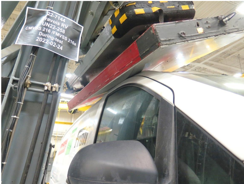
18. Front view with test device on a stop condition
