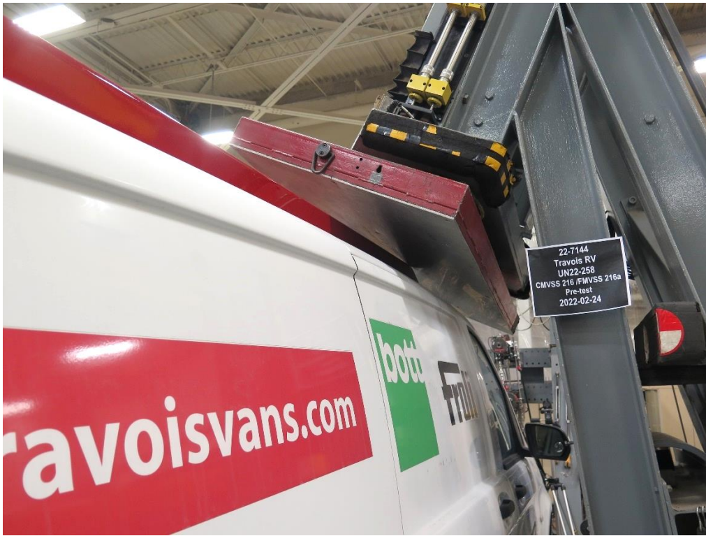
19. Rear view with test device aligned at initial contact point – pre-test
