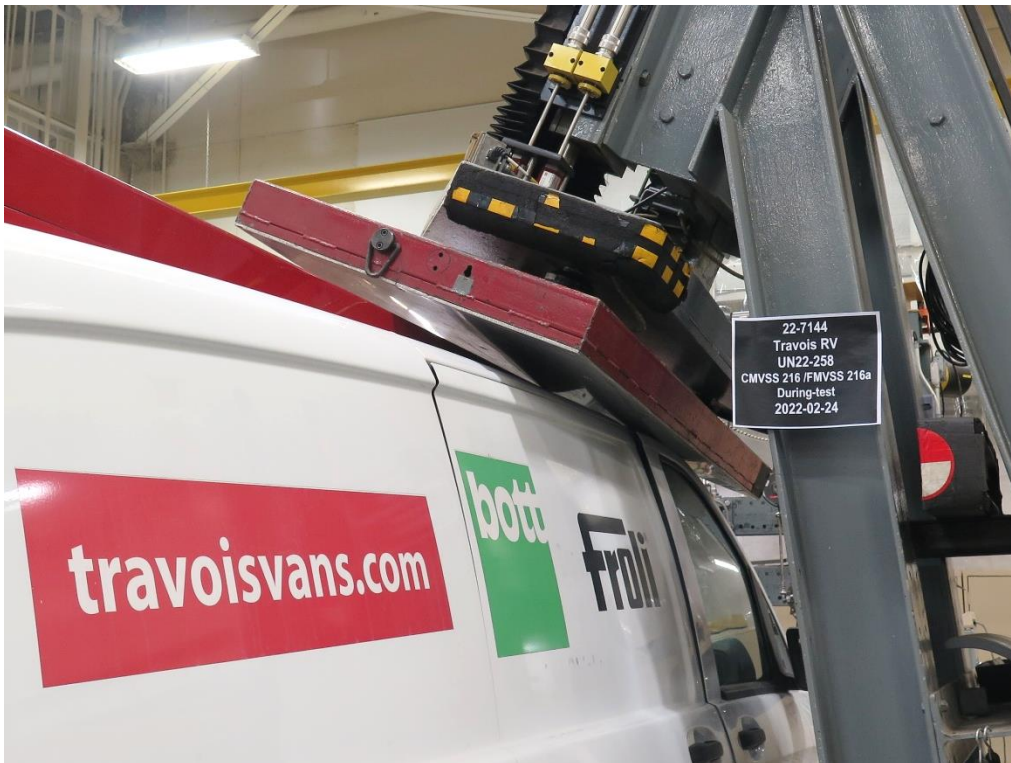
20. Rear view with test device on a stop condition
