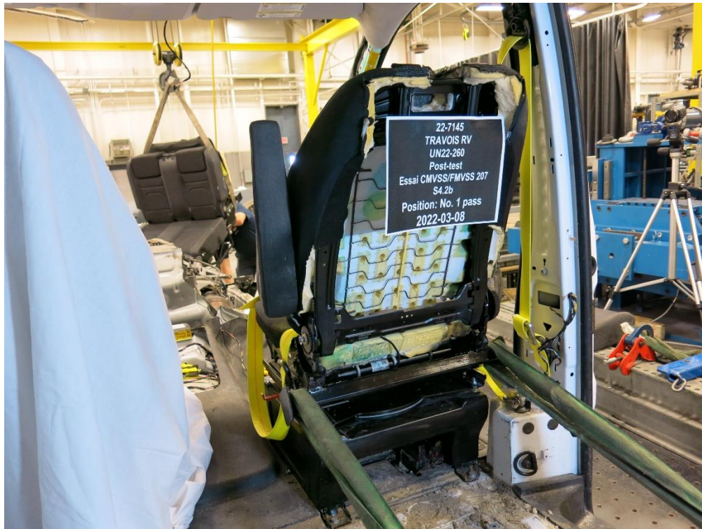
8. S4.2(b) Rearward direction test – post-test
