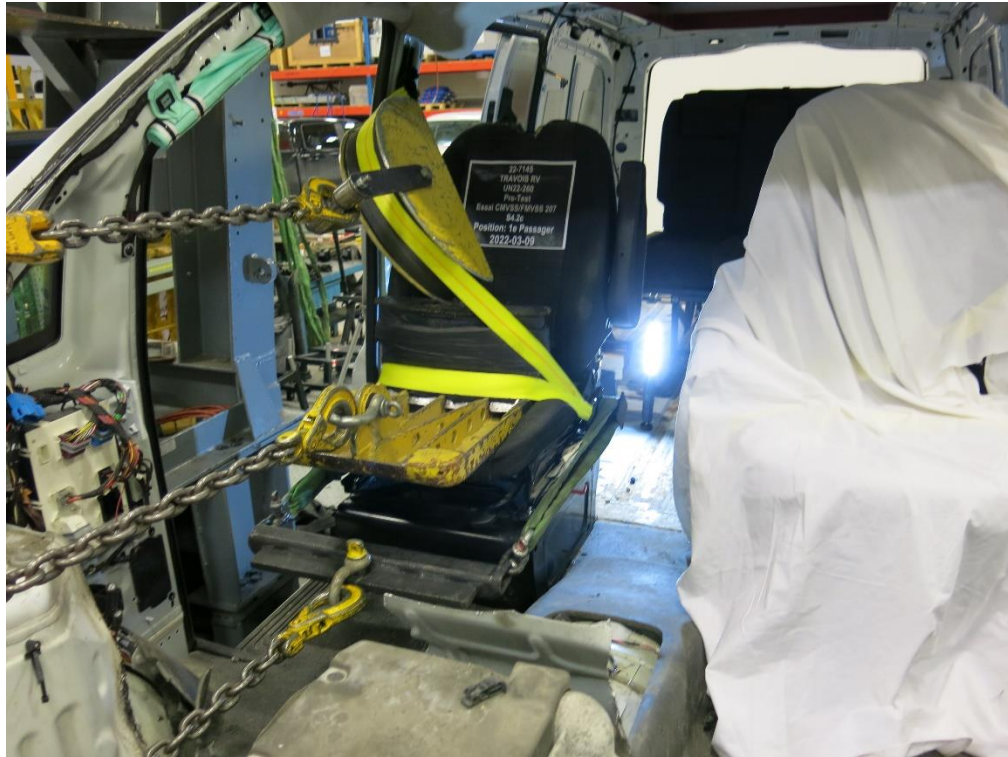
9. S4.2(c) Simultaneous load application test – pre-test
