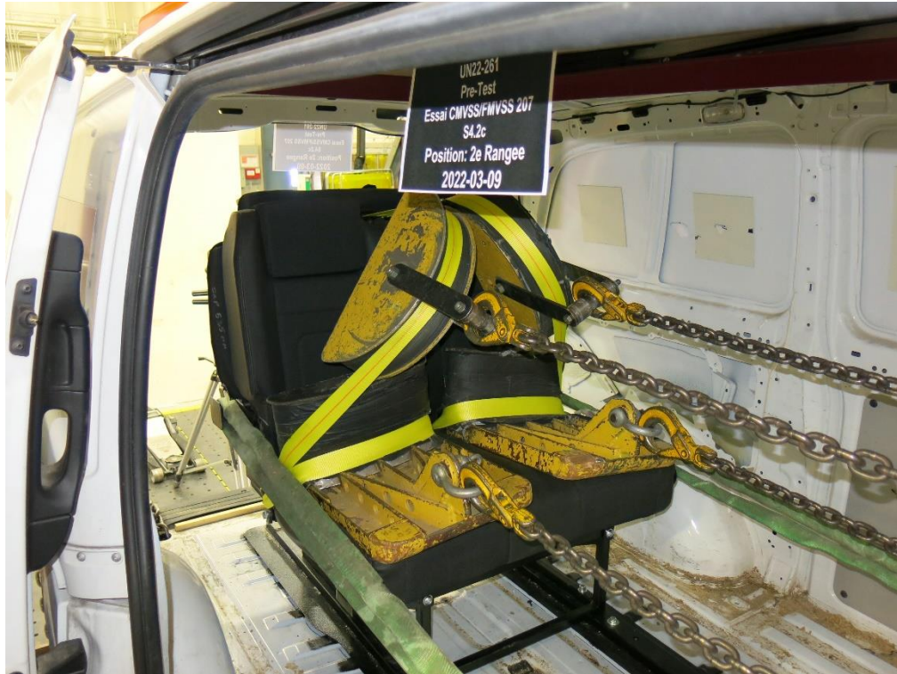
21. S4.2(c) Simultaneous load application test – pre-test
