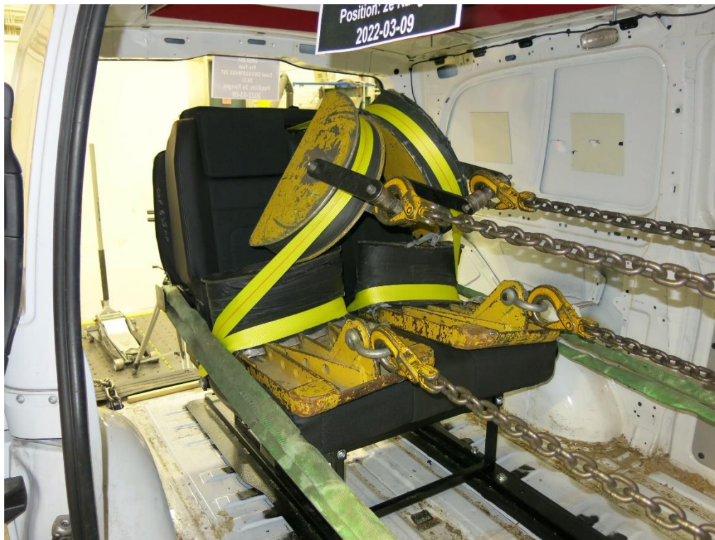
22. S4.2(c) Simultaneous load application test – post-test
