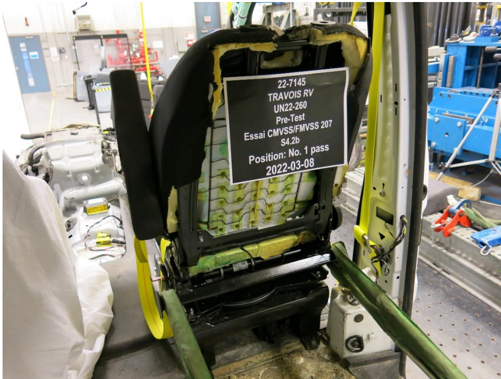
7. S4.2(b) Rearward direction test – pre-test
