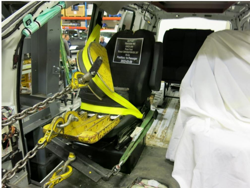
10. S4.2(c) Simultaneous load application test – post-test
