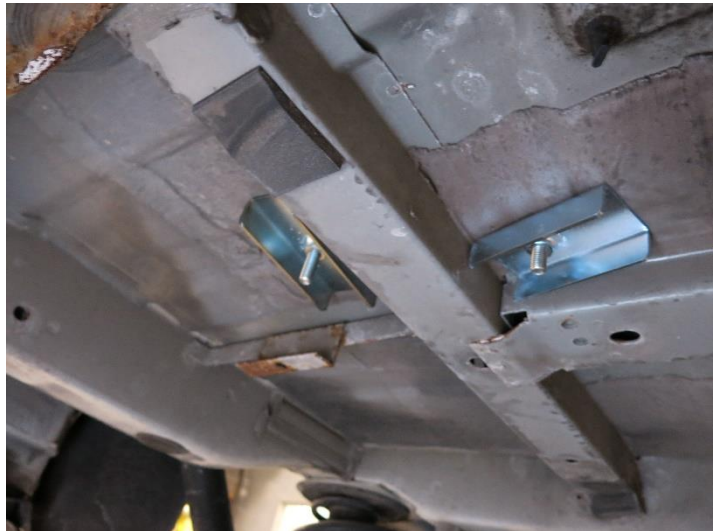
23. Seat anchorages – post-test
