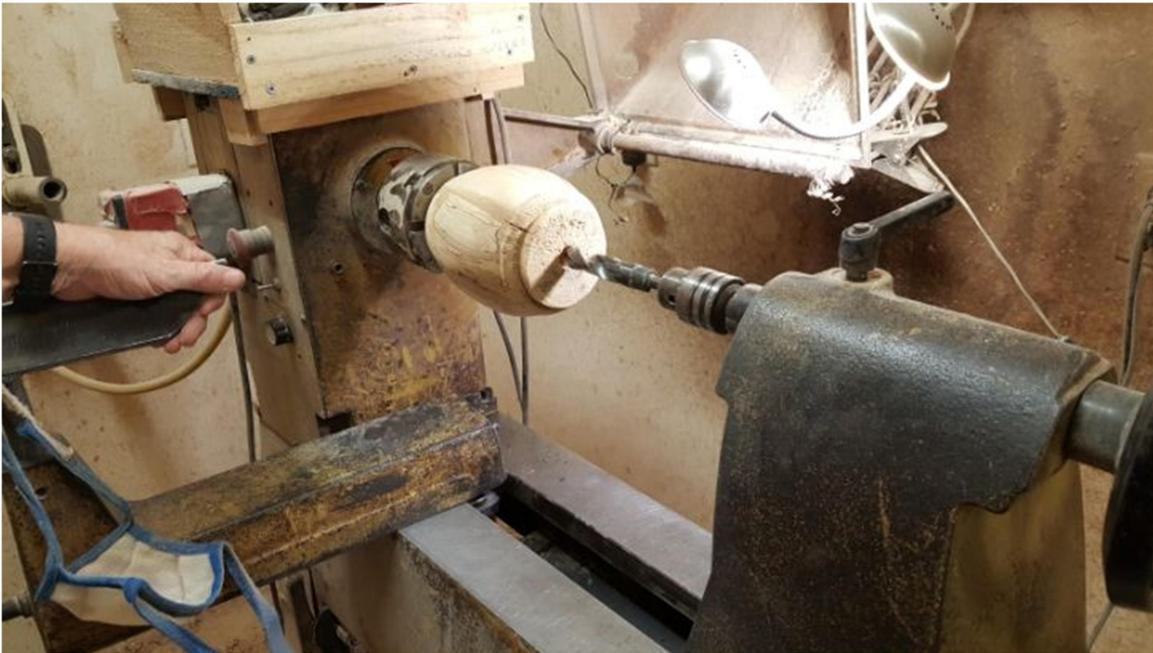
Rechuck the form on the bottom tenon and center up using the tail stock live center and re-bore the hole in the top to eliminate any shrinkage that occurred during the drying process. Flip the form chuck up on the top tenon. Move the live center into the re-bored hole and true up the tenon.
