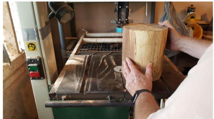
Where possible I like to use the pith as the center of the form. I mark the center and use a compass to draw a circle and use the band saw to cut the blank to the selected diameter. If the height is to be more than 12 inches, I rough turn on the lathe as my band saw will only cut 13 inches in height.
