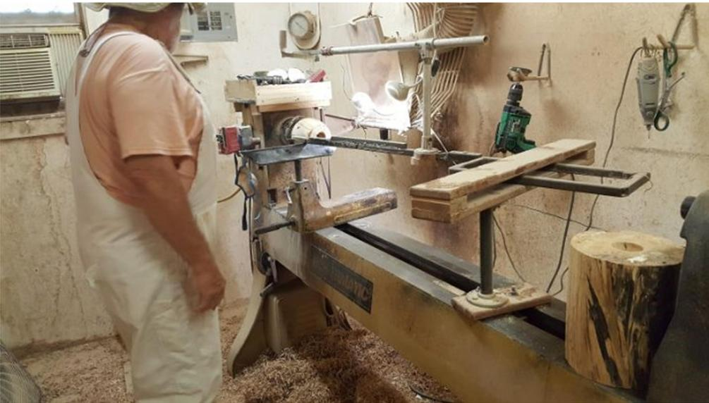
Next I set up my laser guided hollowing rig. The cutter should be as near center as possible, never below center.
