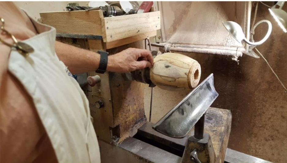
As I near the top of the form I reset the laser to allow at least 1/2 inch thickness in the top. This will give you enough wood to remove the tenon without getting the top of the form too thin. If the form is turned green I remove the form from the lathe and place in a paper bag to dry. The length of time to dry depends on the type of wood. If the moisture content is less than 15% you should be able to return the form to the lathe and finish the form.
