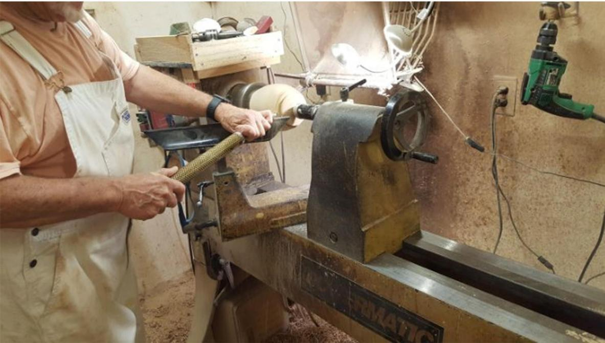
Let the glue dry, then trim and true up the plug on the tenon making sure you leave enough room on the tenon to chuck the form to finish the top.
