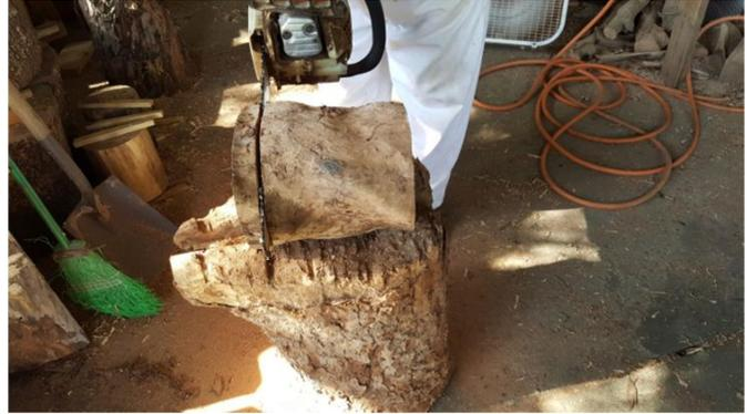
I like to decide what size form I want, select a log that will fit my size requirements. I cut the log to size using these calculations from 10h x 8dia should be cut 12h x 10dia. This will allow for tenons on each end and one inch for the plug material to ensure that you will have a close grain match. The diameter allows the material to be cut or turned to size and hopefully eliminate any voids or other defects which would show up in the side of the form.
