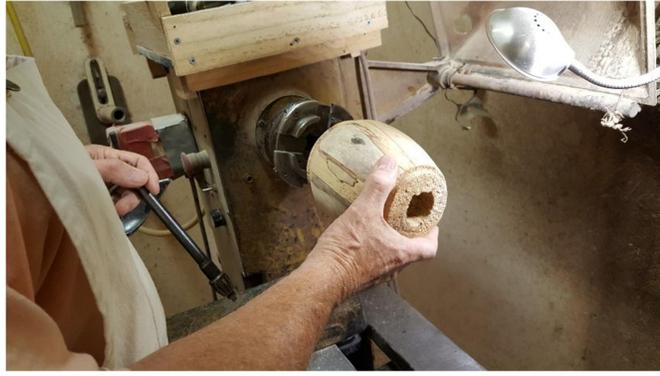
Now I bore out the center using a selected size. My hollow form alignment tools are 1/2, 5/8, 3/4, & 1 inch diameter, so I would use a drill bit the same size as one of those diameters.
