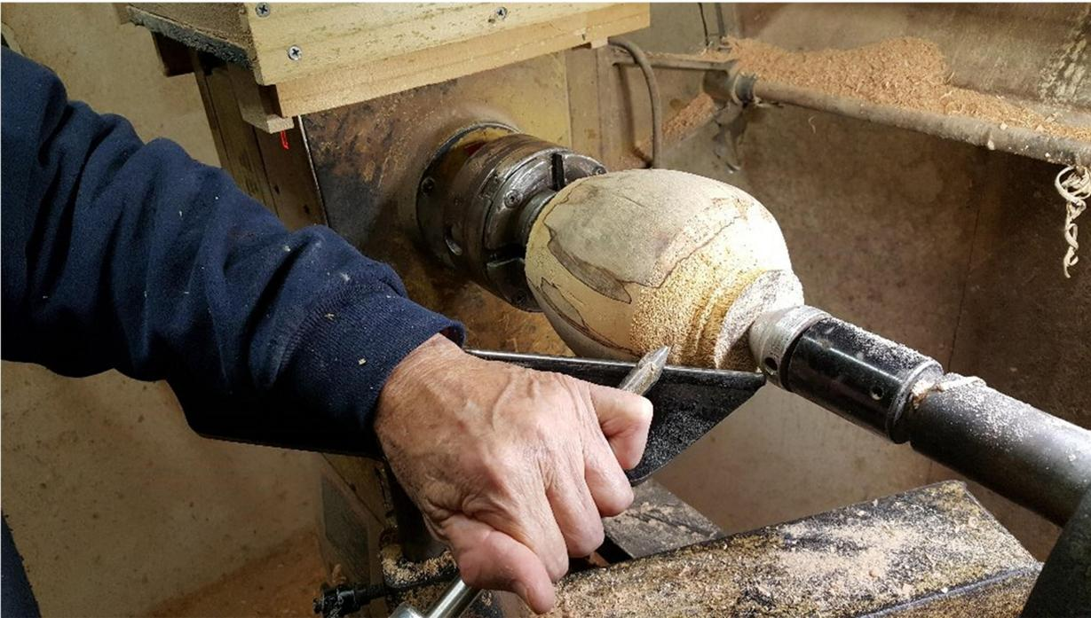
Chuck up the form on the bottom tenon clean up the top of the form to desired shape and sand the top and upper part of the form through your sanding process.
