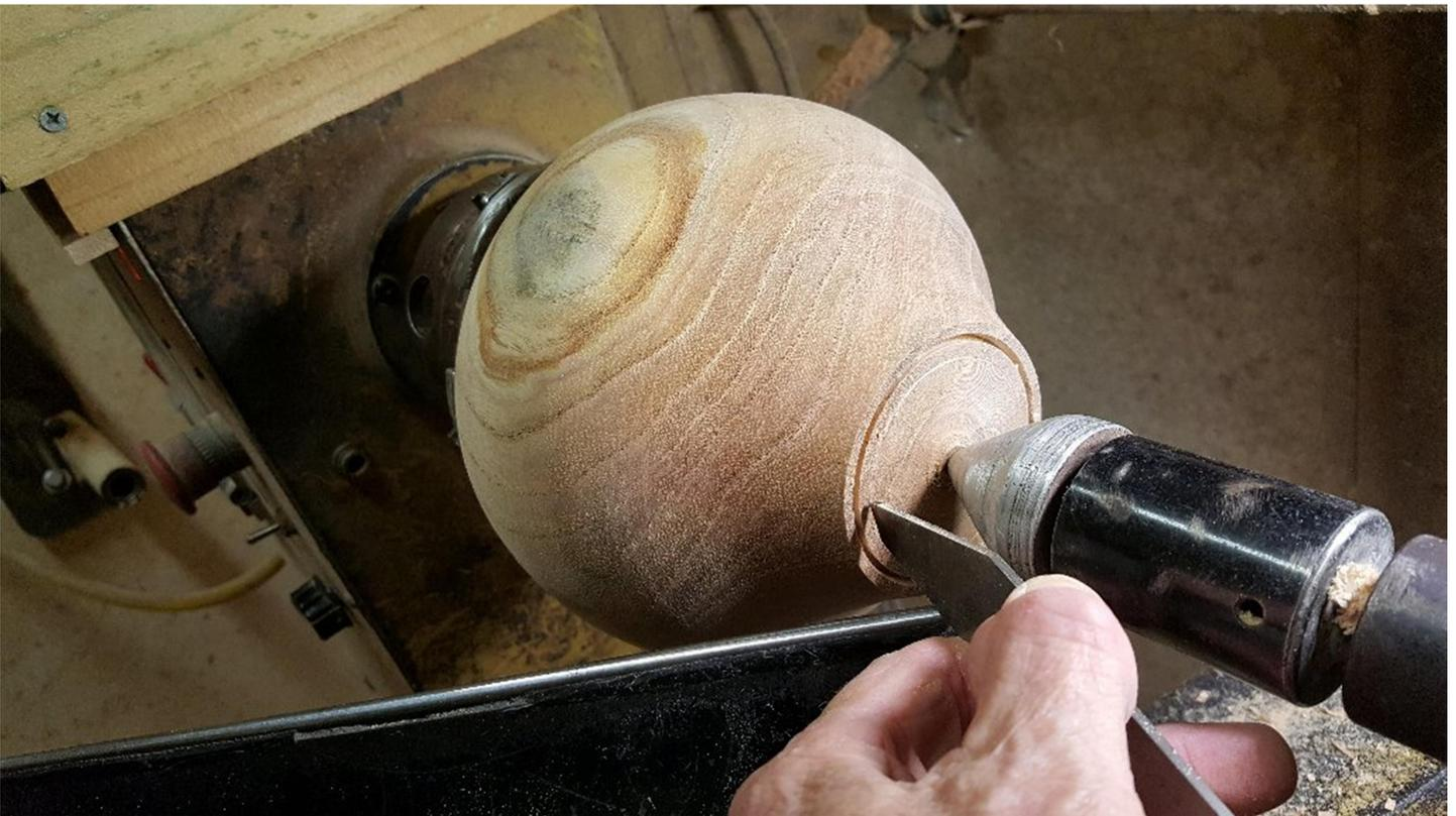
Leave the live center firmed up and use a thin parting tool cut 3 groves 1/8 inch deep in the bottom. Make sure one of the groves is cut over the joint line between the plug and the form.
