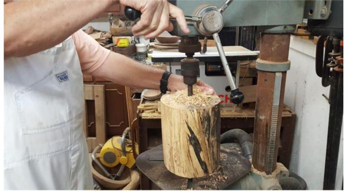
I use a spigot chuck to hold the blank to start turning between centers. It is important to select the end you want on the top of the form as this should show the most figure. The spigot hole will be in the bottom of the form.
