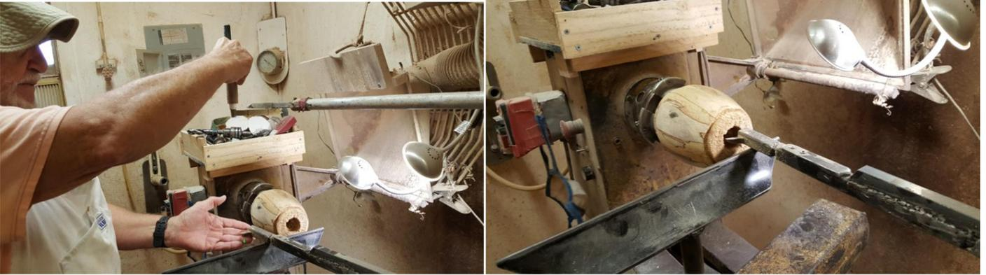
I set the laser to leave between 1/4 - 3/8 inches wood thickness in the sides of the form. It is important to leave at least 1/2 inch thickness in the bottom so the plug will have enough wood to cut groves 1/8 inch deep and have enough wood left to connect the plug to the form. Next hollow out the form. I stop and check the laser alignment frequently to make sure the laser remains aligned and check that the chuck remains tight on the form.
