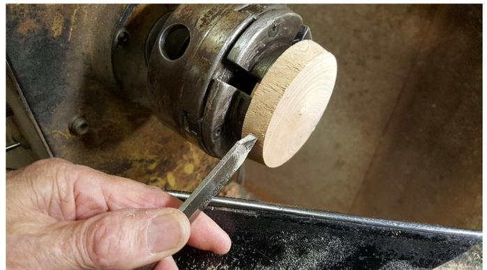
The opening in the bottom should be cut at a slight inward angle so as to fit the plug which has been cut at a slight inward angle to form a wedge. The wedge shape will prevent the plug from slipping through if you cut it a little small. Super glue the plug and slip it into the opening in the bottom.
