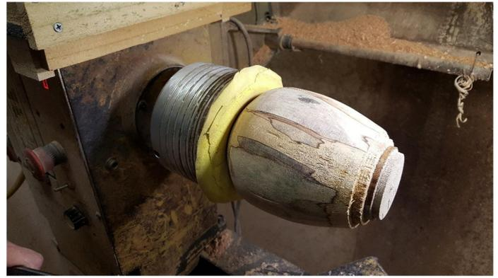
Flip the form and vacuum chuck or jam chuck the form using the alignment tool, firm up the live center on the center of the plug to ensure the form remains in place. Shape the bottom by cutting the tenon off.
