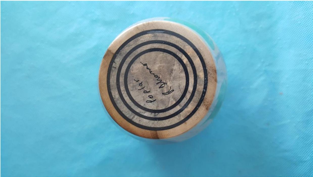
Remove the form, fill the grooves with epoxy, let dry for 48 hours and vacuum or jam , sand off the excess epoxy and the lower part of the form using your sanding process.
