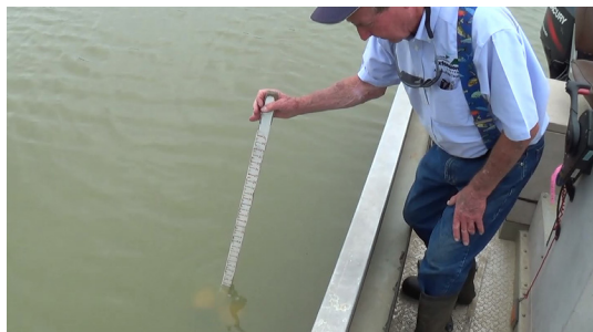
Lowering a Secchi disc to measure water transparency
