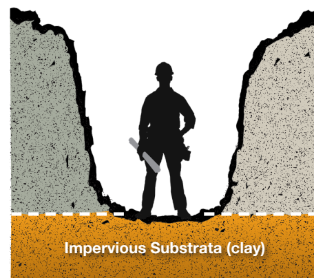
Cutting a trench for the clay core of the pond.
