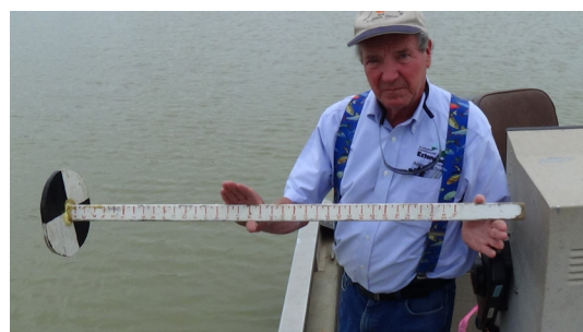
A Secchi disc can be used to determine when to fertilize.
