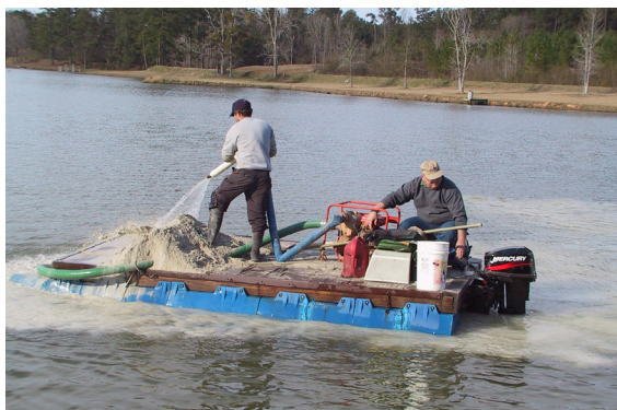
Lime application using a pontoon barge and water pump to evenly distribute the lime.
