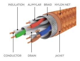
Pure Oxygen-free Copper Conductors Super Flexiable FMPE+SKIN Insulation Aluminum Mylar Coverage >100% Aluminum-magnesium Alloy Shielding Antifriction Nylon Mesh Fabric
