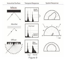
surfaces. Following the introduction of quantifiable reflection phase gratings by RPG Diffusor Systems in 1983, diffusers have continued to evolve and are now used as a complement to absorbing surfaces. At this time, there is a full complement of diffusing surface topologies to be included in contemporary architecture (www.rpgacoustics.com). While absorbing surfaces attenuate
