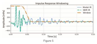
this reason, we suggested in the RFZ control room design in 1996 that the loudspeakers be flush mounted. We can estimate the SBIR in the NIRO program, which we will describe later, by windowing the early part of the room's impulse response, as seen in Figure 5.
