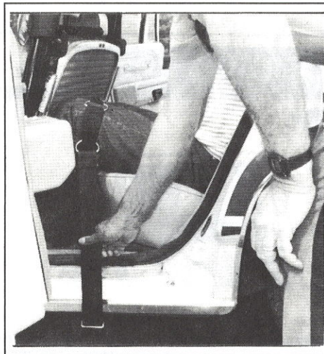
Pull door belt toward door and place belt end labeled "this end out door", over rocker panel.
