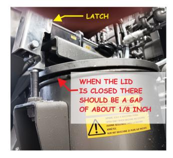
It is extremely important that when the button trap lid is closed (NOT LATCHED) there is about a 1/8" gap with the lid resting on the handle knob. When the lid is latched this gap will close and pressure will be applied through the handle securing this strainer in place. If the strainer is not seated properly the strainer will tend to float off its seat, allowing unwanted lint and debris to infiltrate the suction side of the solvent pump.
