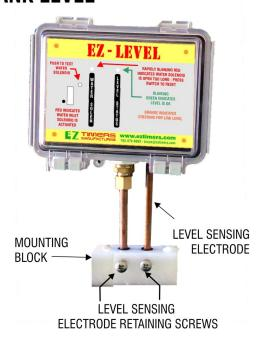
**STEP 2:** Shortly after turning power on to the EZ LEVEL the indicator light labeled LEVEL STATUS should be glowing orange indicating that a low level has been sensed. After a few seconds indicator light labeled WATER SOLN will glow red indicating that the Water Inlet Solenoid has been energized, allowing make up water to flow into the return tank and begin the filling process.
