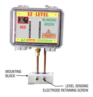
**STEP 4:** Slide the entire EZ LEVEL down through the holes in the Mounting Block until the it is about an inch above the Mounting Block. The EZ LEVEL can slide up and down through the Mounting Block to adjust the water level height in the return tank. When the desired water level is determined secure the adjustment by screwing in the Retaining Screws until they firmly hold the EZ LEVEL in place.
