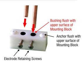
$\ensuremath{\mathbf{STEP}}$  3: Slide the Electrodes through the holes in the Mounting Block.
