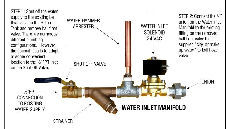
STEP 3: Once all the connections are made and tightened close the Shut off Valve on the Water Supply Manifold and turn on the water supply to the manifold. After the water is turned on slowly open the Shut off Valve, there may be a short surge of water thought the Water Inlet Solenoid. Check for leaks.
