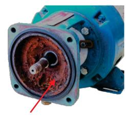
BUILD UP OF SCALE BEHIND PUMP IMPELLER
