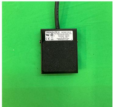
In many cases the screw holes used for mounting the new switch is not sized correctly for the old mounting screws. You can drill larger holes or I 4 have found the easiest solution is to use silicone sealant to cement the switch in place overnight.
