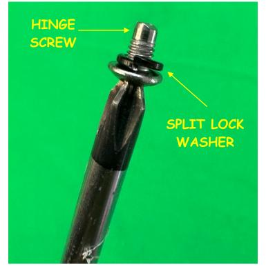
STEP 12: Place the split lock washer on the hinge screw.
