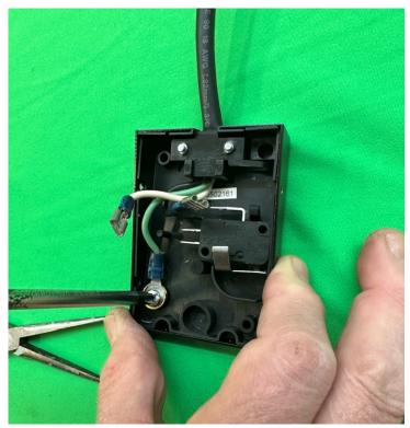
STEP 5: Unscrew the ground wire connection from the switch body.
