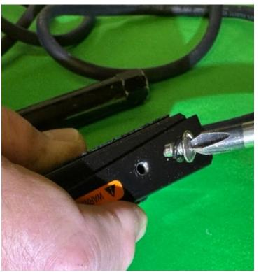
STEP 14: Insert and firmly tighten the hinge screws. HOORAY, JOB DONE!
