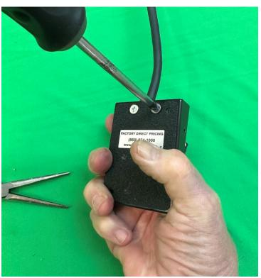
STEP 6: On the bottom of the switch body, unscrew the two screws from the strain relief clamp.
