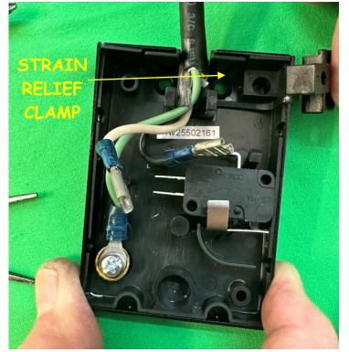
STEP 7: Turn the switch over, open the strain relief clamp, and remove the wire.
