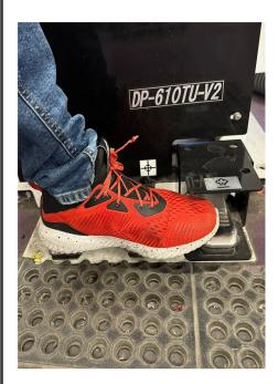
STEP 2: step on the buck steam and vacuum valve simultaneously to bleed off any remaining steam pressure.
