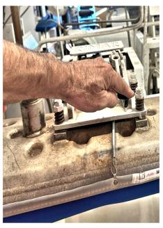
STEP 1: Shut off the steam and return valves. Close and lock the head. Then press down the head steam valve while preforming STEP 2.
