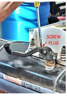
Try screwing the screw plug into the valve handle to stop the leak before performing further repairs. (NOTE-ON SOME VALVE HANDLES THERE IS AN ALLEN SCREW RETAINING THE PLUG)
