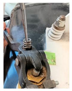
STEP 5: Remove the spring from the head valve. A needle nosed pliers is useful for this task.
