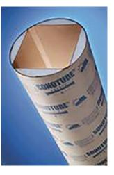
It is recommended to use Sonotube® filled with foundation grade high strength concrete with steel rods enforcement, 30" deep or 4" deeper than local frost line.
