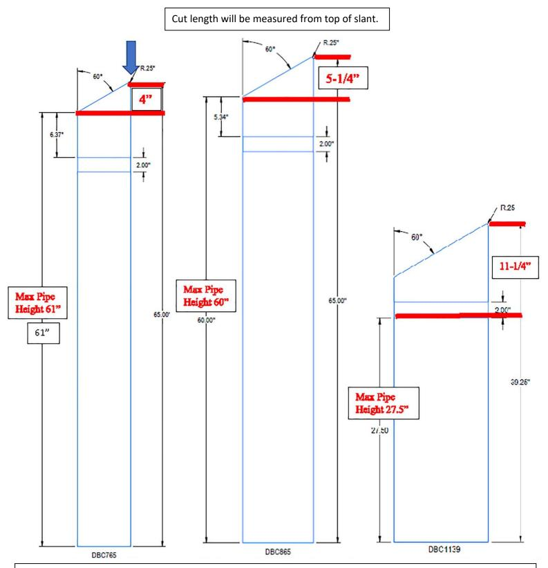
Cut length will be measured from the top of the slant. Keep this in mind when asking us to cut the decorative covers, as cut covers are not returnable. Max pipe heights are noted above and will need to have the "slant" measurement added to them to get the cut length. Box dims will be 1" taller than cut length.
