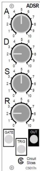
The Circuit Slices ADSR module is a re-triggerable envelope generator for modular Eurorack-compatible synthesizers. This popular module has been revised (part number CS017n) with a standard 6 HP front panel.
