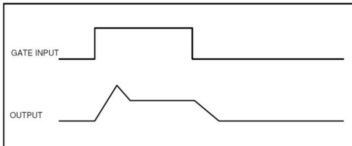
A Gate input accompanied with multiple triggers will produce the following response:
