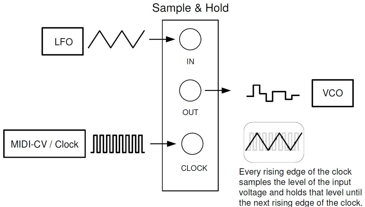
If your clock signal is generated from a MIDI-CV module having a MIDI clock output, your patch will be in sync with your MIDI drum machine or computer sequencer. This is not the only patch to try. As an example, the gate from an analog sequencer could be divided by 4, using a clock divider, and sent to the S&H CLOCK input allowing you to produce a CV that ‘holds’ and only changes for every fourth note played.
