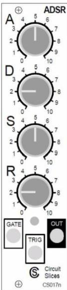
The Circuit Slices ADSR module is a re-triggerable envelope generator for modular Eurorack-compatible synthesizers. This popular module has been revised (V4) to include a jumper option to limit the output to 5V, which allows the module to be used with a wider variety of systems. The front panel includes a green LED that indicates the state of the output.
