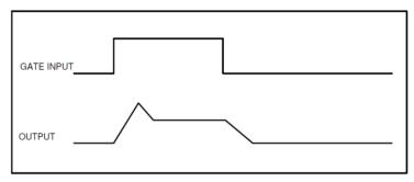
(note that the attack, decay, and release lines will show as curves on an oscilloscope – the changes are exponential.)
