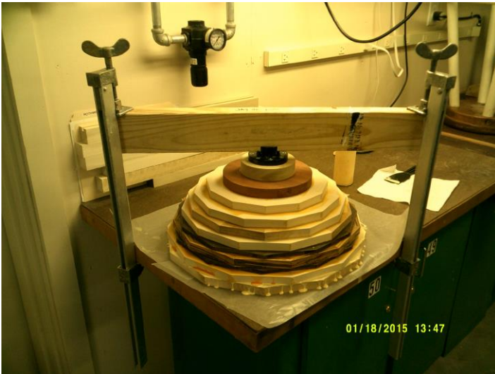
Creative clamping to achieve proper pressure
