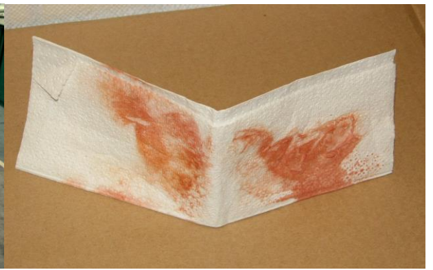
Residue after acetone wipe
